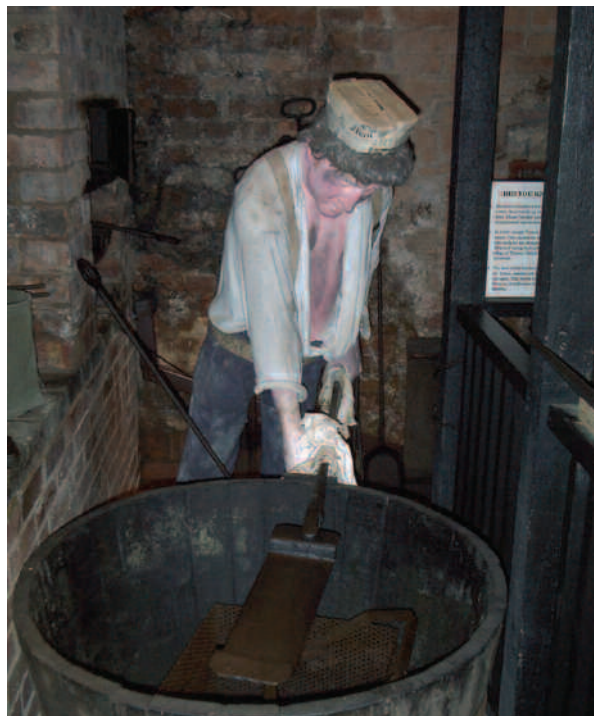
FAR LEFT: A needle pointer at work. Pointing the needles was the most dangerous job in the needle-making industry. LEFT: A needle hardener at work. The needles were hardened and tempered before being sent to the scouring mill. Photographs courtesy of the Forge Mill Needle Museum, Redditch, Worcestershire, England.
